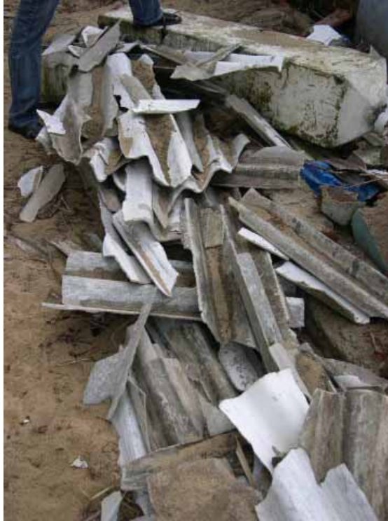
Dangerous waste. Asbestos rubble poses a great health risk.
